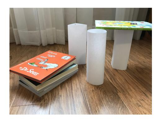
Get three pieces of paper and using tape, fold each one into a different paper tube shape - a circle, a square, and a triangle. Guess which shape is the strongest and then try it out by stacking books on each one.
