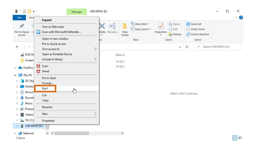
You can also eject flashdrives or external harddrives by clicking on the arrow in the bottom-right corner of the screen and right-clicking on the **Hardware** icon. Then, click on the **Eject** prompt next to your device in the list.
