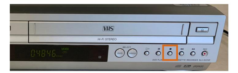
When you are finished scanning your tape, be sure to press the **Rewind** button to rewind your tape. When the tape is finished rewinding, then you can press the **Eject** button to retrieve your tape.
