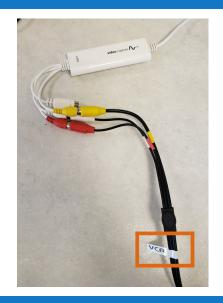
Next, make sure the VCR is connected to the Elgato Video Capture device.
