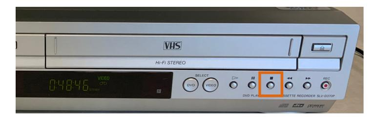
When you are finished scanning your tape, be sure to press the **Rewind** button to rewind your tape. When the tape is finished rewinding, then you can press the **Eject** button to retrieve your tape.
