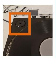
After you've placed your record onto the turntable, press the 33 or 45 button in the bottom left, to correspond with your record size. Press both if your record plays at 78rpm.
