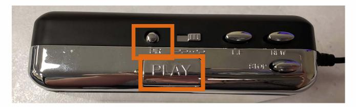
When you're done, press stop in Audacity. If you did not finish side B you can press F.F. (Fast Forward) to bring the tape to the end. This means Side A is rewound and ready for its next use.
