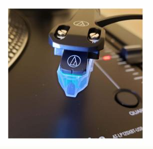
Remove the protective sleeve of the needle by sliding it towards you.
