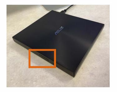
When you are ready to burn your CD open the disk drive by pressing the button on the front, and inserting your CD. Make sure that it is a CD-R and not a DVD-R.
