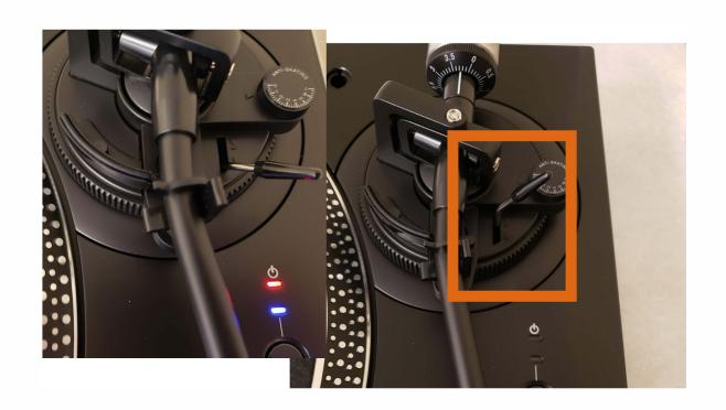
Ensure the lever that controls the needle's height is in its upwards (raised) position. At this point you can press the 'Start/Stop' button in the bottom left. Your record will now begin to spin.
